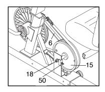
(15). To tighten the Drive Belt, turn the two Drive Belt Adjustment Nuts (50) clockwise; to loosen the Belt, turn the Nuts counterclockwise. Make sure that the Flywheel is straight and tighten the 5/16" Nylon Jam Nuts (18). Reattach the side shields and pedals.
